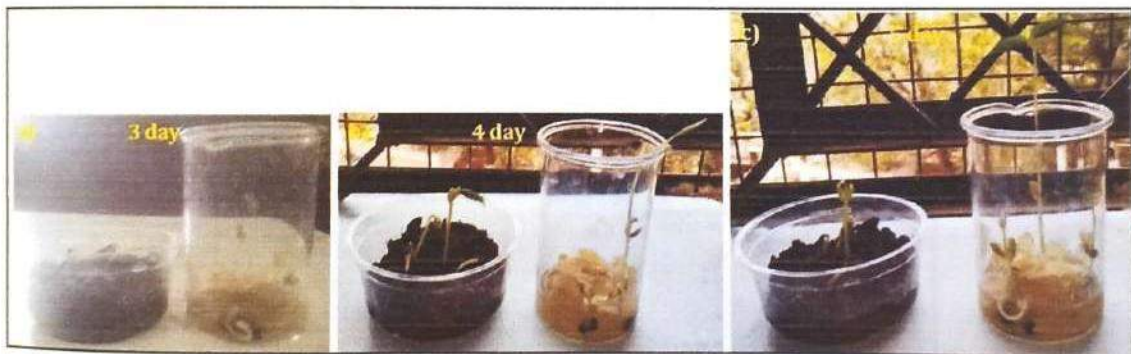
Figure 3.3: a) After 3 rd day b) 4 th day and c) 5 th day seed germination of bioepoxy resin CA as a plant growth substrate compared with soil.
